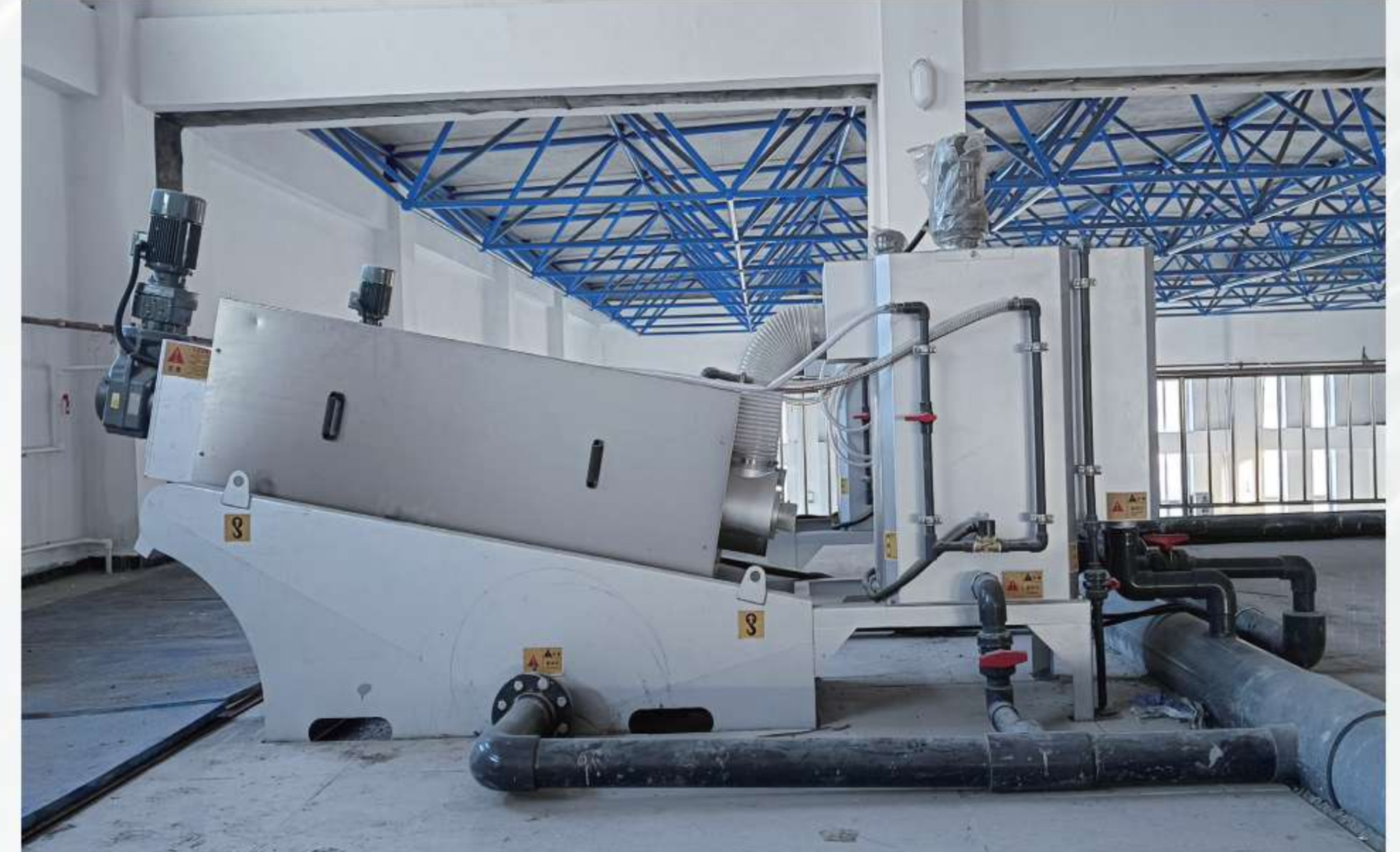
Screw-type sludge dewatering machine
