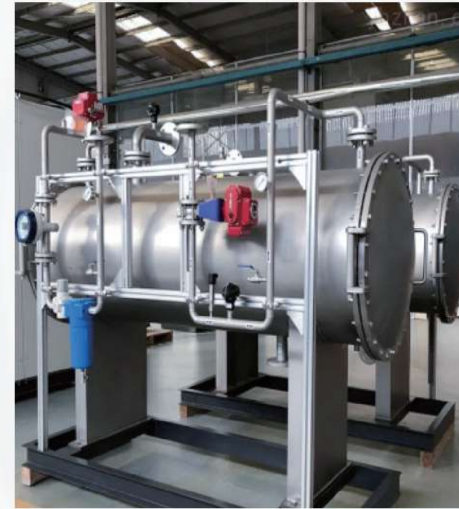
Ozone disinfection equipment
